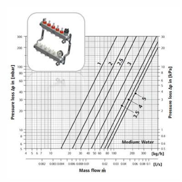
Flow and pressure loss in [mbar] and associated correlating [kPa] is indicated in the attached chart. The unit has the ability to adjust flow in accordance with professionally design project criteria. The flow meter is adjusted using the anti-clockwise and clockwise trunich mechanism to open and close the port and increase and reduce flow respectively.
