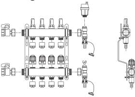
When initially filling the UFH heating system it is important to remove the air in the pipework. In order to do this a hose should be connected to the upperfill valve and the bottom valve should be opened to allow the water to be flushed into a bucket or drain.
