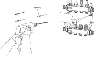
Make sure that the manifold is level and that it is high enough so that the pipes can be installed easily.
