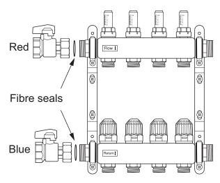
Fit the end connection with the manual air vent and blue handled drain/filling valve to the return manifold and the end connection with the manual air vent and red handled drain/filling valve to the flow manifold, using the fibre seals provided.
