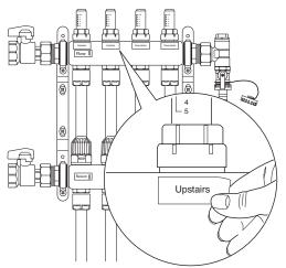
Fit the blue handled 1" union ball valve to the return manifold and the red handled 1" union ball valve to the flow manifold using the fibre seals provided.
